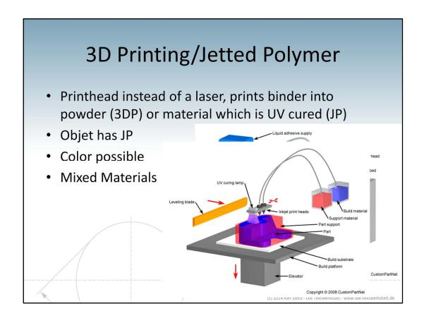
Then there are several similar technologies involving something like inkjet printheads. The ZPrinters print colored printer into a powder material which makes it possible to print full color, gypsum-like parts. Jetted polymer means that the material itself is coming out of the printhead. Objet uses this to generate Digital Materials, that means they print different materials instead of different colours. This makes it possible to influence for example the stiffness of a rubber-like material.
