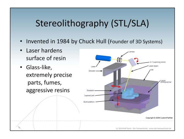
The oldest technology is Stereolithography. It was invented in 1984 by the founder of 3D systems, Chuck Hall. The technology is using a laser beam that is directed by this mirror. The laser beam draws the first layer on the surface of a resin that is in this basin. The resin hardens instantly when it is touched by the Laser light. After a layer is drawn, the build platform goes down one layer height and the next layer is printed.
