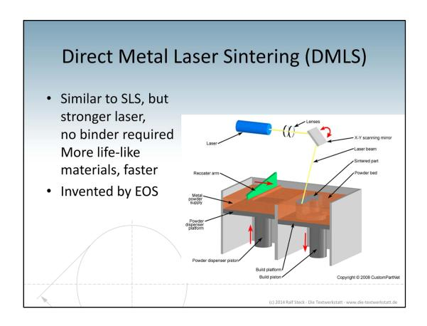
If you use a more powerful laser, you can melt metal powder directly. This has the big advantage that real-world materials like stainless steel can be used. And it's faster because the burning is removed. By the way, this technology was invented by EOS, a company from Gräfelfing, here in Munich.
