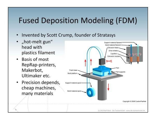
The last and, when it comes to cheap 3D printing, the most important technology is Fused Deposition Printing. Scott Crump invented it literally when he played with a hot-melt gun. It's exactly that: Plastics filament is fed into a moving, hot nozzle that lays a bead of plastics on the print platform. It's really easy to build such a printer so most of the cheap printers are using this technology, even if it's not as precise as other technologies.
