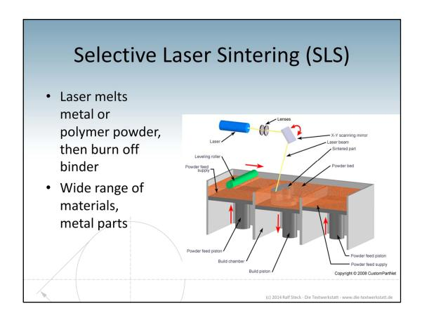
Next we have Selective Laser Sintering, SLS. This also uses a laser, but not a resin. The material is binder-coated plastics or metal powder. The laser melts the binder-coated particles together, after every layer the build platform goes down and a recoater puts the next layer of powder on top of the already printed part. After the printing process, the part is put into an oven and baked together at about 900 degrees Celsius.
