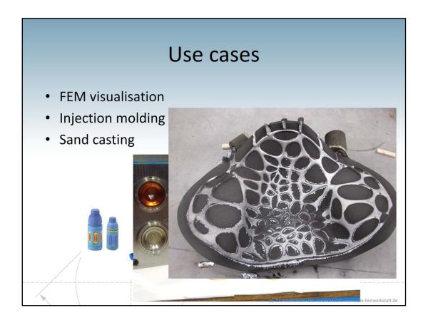
The third use case are using 3D printing in a more indirect way, for example to show the stress in parts as simulated in a FEM computation. Very new is a material that can be used to print injection molds. In the foreground you see prototype membranes casted in the green molds. So it's possible to evaluate the casting process before you make the very expensive production molds you see in the background.
