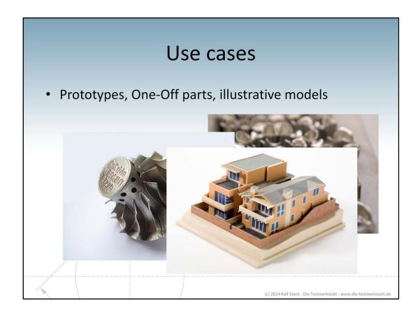
The first use case and where the technology comes from are prototypes, One-Offs or illustrative models. 3D printing is more or less useless for mass production, but when it comes to parts you need relatively fast and just one or a few, it's unbeatable. Another thing is Rapid manufacturing, this means mass production if individualized products.
